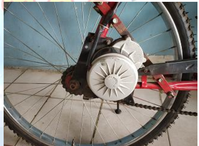
Fig. 1 Hub motor attached to Back wheel
