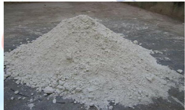
Figure 3.1.1 : PAPER WASTE SLUDGE
