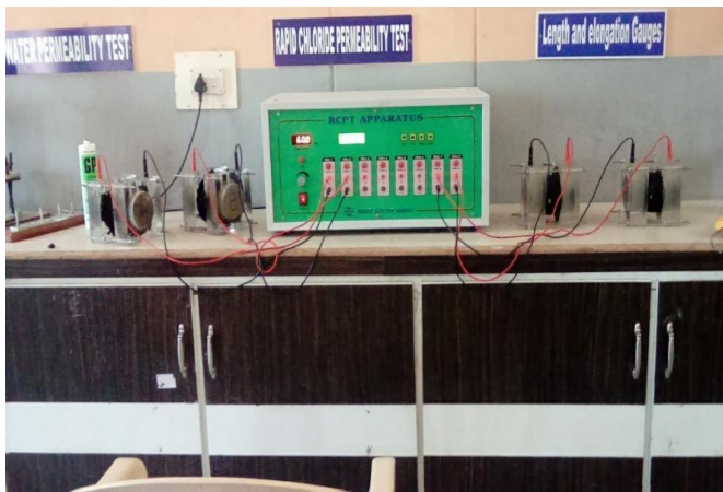
Fig. 5.4.1 : Rapid chloride permeability test setup
