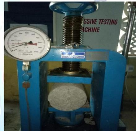
$$\text{Spilt tensile strength } T_{sp} = 2P / \pi DL$$
