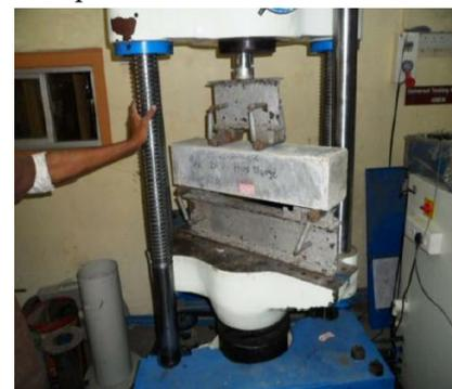
$$\text{Flexural strength } (f_b) = P \times L / b \times d^2$$
