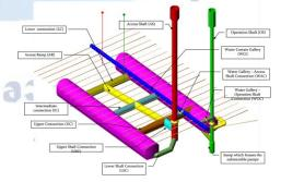
**MANGALORE:**The Mangalore project is located over an area of 104.73 Acres the total approved cost Rs.1227 crores the storage capacity 1.5MMT (11MMbbl) it is constructed four parallel caverns tow of them area 913m long and two 873 m long the cavern width is 20 m with a maximum height of 31 m. the total tunneling including shafts of Mangalore facility exceeds 9.2km. It is tow compartments required each compartment commencement of construction April, 2009.
