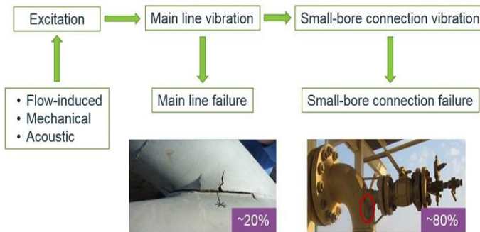
Figure 2: Mechanism of induced vibration
