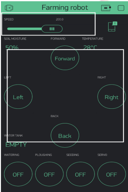
Figure -12: Directional Buttons and Speed Control in the Blynk app.
