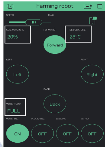
Figure -13: Display Details of Temperature, Soil Moisture and Water Level in the Blynk app.
