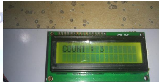
Figure 11: LCD display when there are 3 persons inside the room
