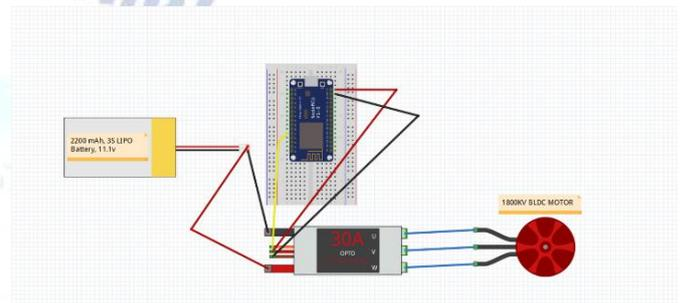
**Figure 3: Brushless Motor Interfacing with Nodemcu**
