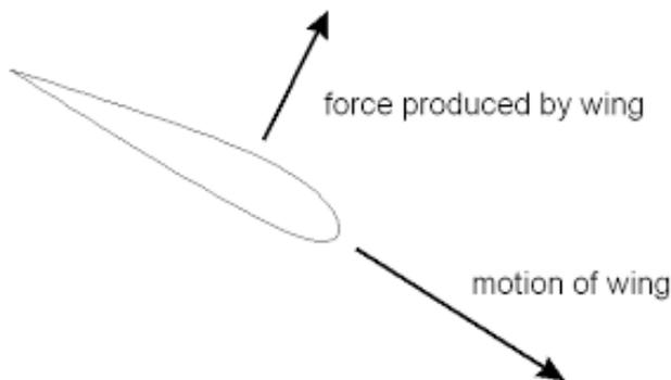
**Figure 2: Principle reflects to wing mechanism**
