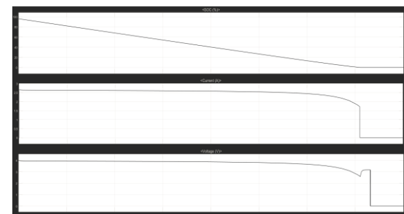
Figure 3 complete discharging of battery
