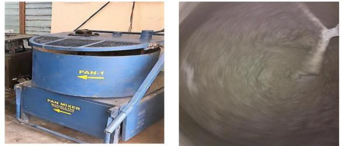
Figure 2: Mixing of concrete in Pan Mixer
