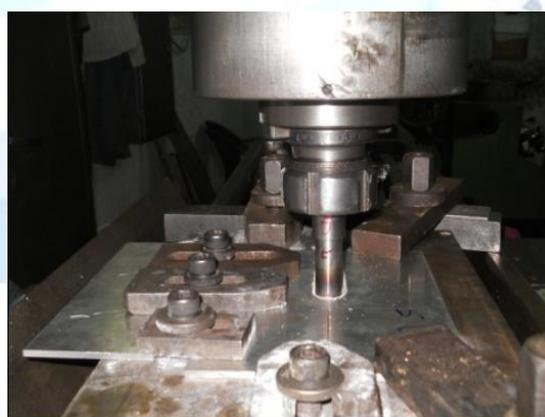
Figure 1 Friction stir welding experimental set-up
