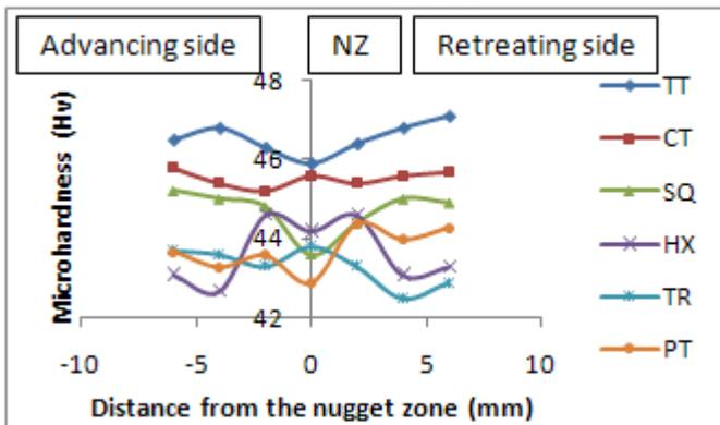
Figure 3 Micro hardness distribution of FSW joints for different pin profiles
