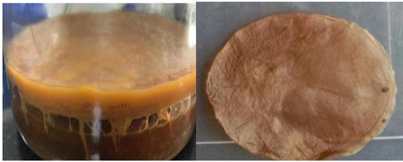
Figure 1. (a) BC sheet formed in a glass tank and (b) Dried BC film.
