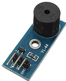
Figure -10: Pin out Diagram of Passive Buzzer
