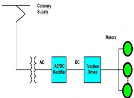
Figure-1 Supply unit of locomotive.
