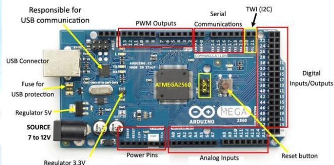
Figure-2 Arduino mega 2560
