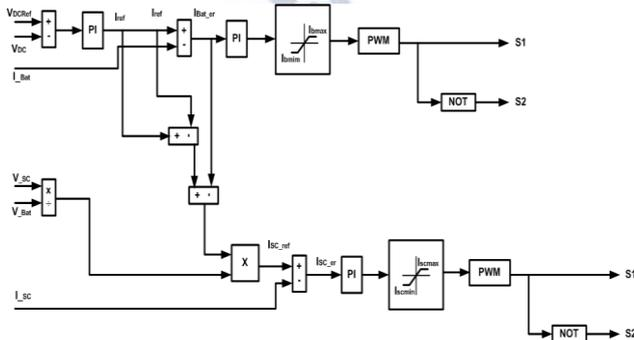
**Fig 5: Control Circuits of parallel operation of ESS**
