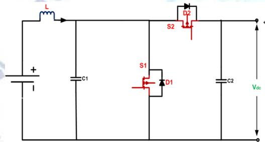
**Fig 4: Bidirectional DC/DC converter of Battery and Super capacitor**
