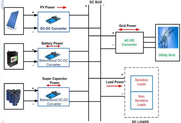
**Fig. 1. Block Diagram for power management strategy in a hybrid DC microgrid**
