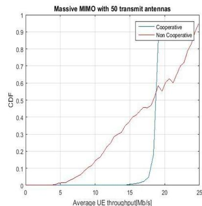
Fig.4. UE throughputs CDF for non-cooperative and cooperative massive MIMO with 50 transmit antennas
