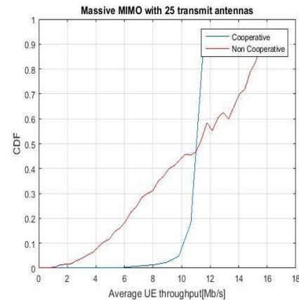
Fig.3. UE throughput CDF for non-cooperative and cooperative massive MIMO with 25 transmit antennas.
