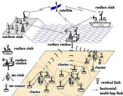
**Fig 1. Underwater Sensor Network Architecture**
