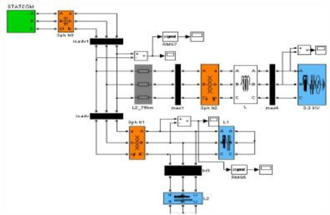
Figure6. Circuit diagram with STATCOM model
