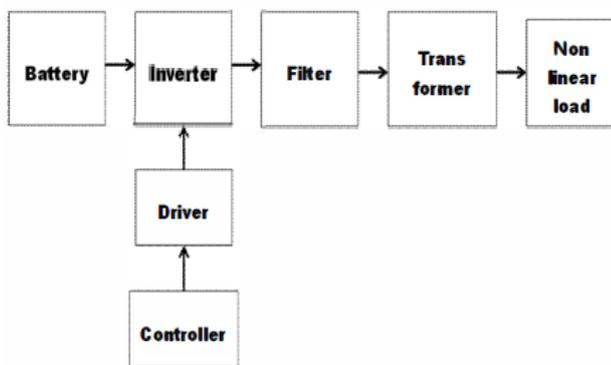
Figure 19.Hardware implementation block diagram
