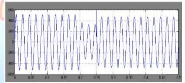
Figure 8.Load voltage with sag conditions
