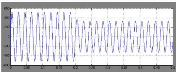
Figure 12. Load voltage with sag conditions
