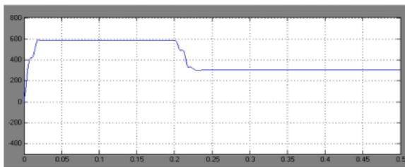
Figure5. RMS Load voltage with sag conditions
