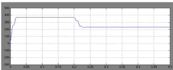
Figure 13. RMS Load voltage with sag conditions
