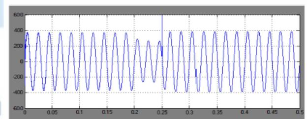
Figure 17. Load voltage with sag conditions
