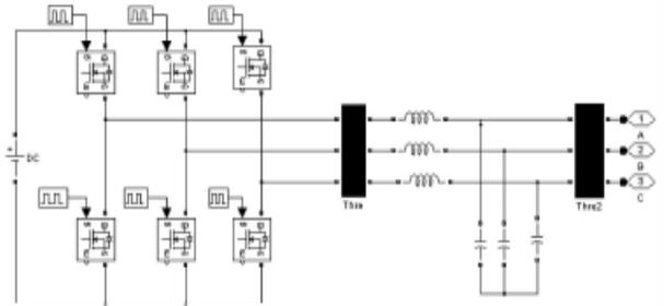
Figure 14. STATCOM circuit diagram
