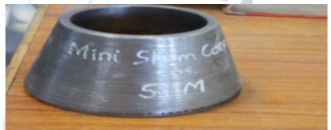
Figure No. 2 – Mini slump cone
