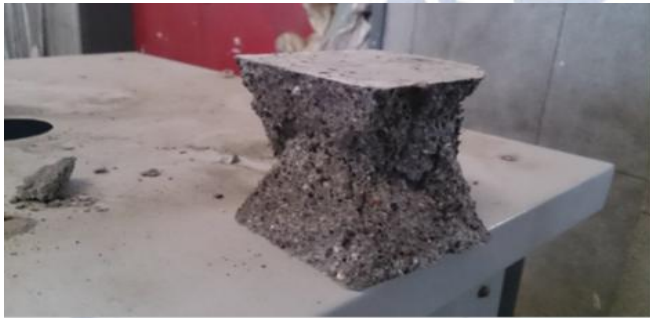
Figure No. 5 – Failure pattern of cube
