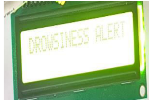
Fig 8: LCD Indication of Driver Drowsiness Detection The LCD displays a “Drowsiness Alert” message when fatigue is detected, notifying the driver in real time.
