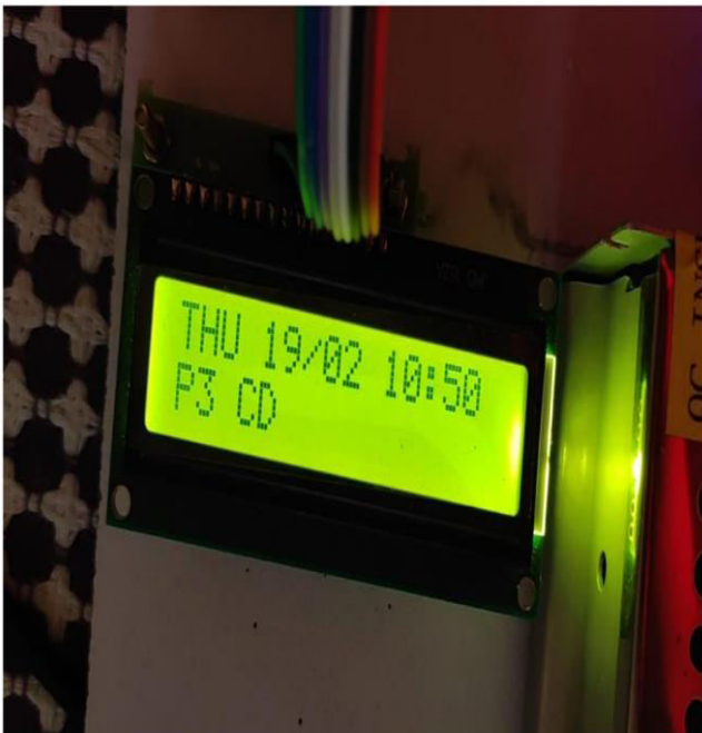
Fig 4: LCD Display Showing Date and Time Information This figure shows the LCD display module that provides real-time information such as date, time, and system status using the RTC module. When an RFID card is scanned, the system verifies the data and records attendance. The LCD then displays confirmation, making the system user-friendly and efficient for monitoring.
