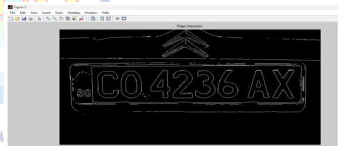
Figure 8: Edge Detection using Canny Operator
