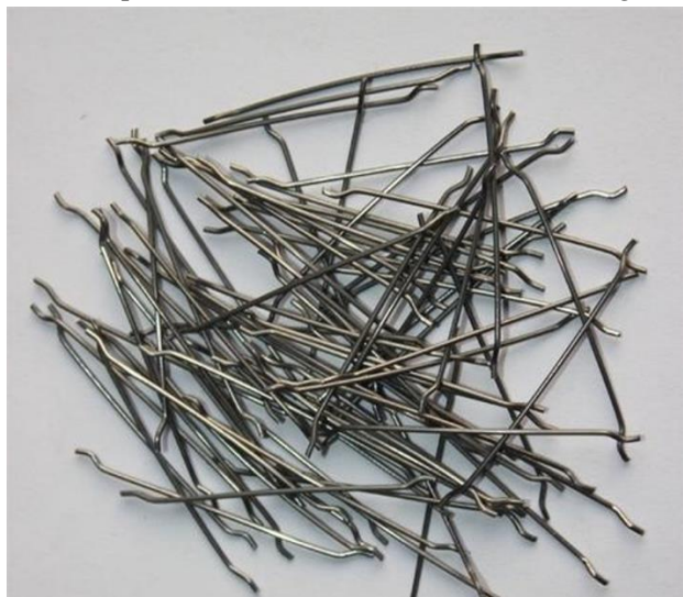
Figure 1. Steel fibers used in the experimental programme
