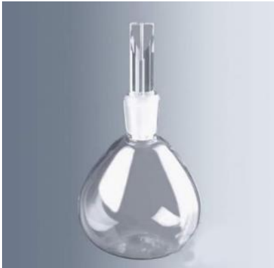
Figure 2. Specific-gravity bottle/apparatus used in the preliminary material investigation
