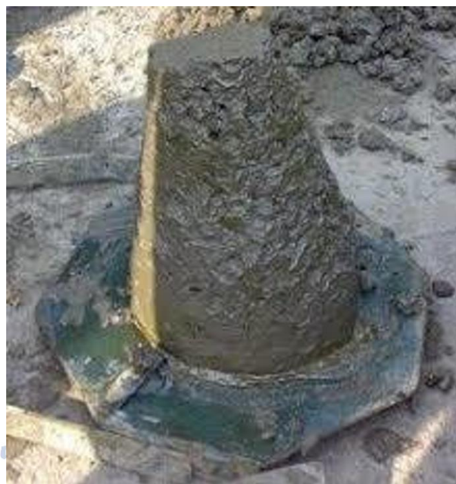
Figure 4. Slump-test photograph from the source experimental study.
