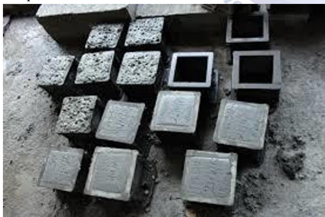
Figure 3. Cast pervious-concrete cube specimens (source document photograph).
