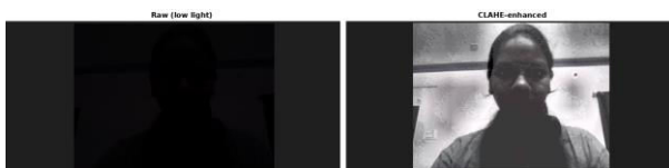
Fig-8: Low-Light Preprocessing - Raw Frame (Left) vs. CLAHE-Enhanced Frame (Right)
