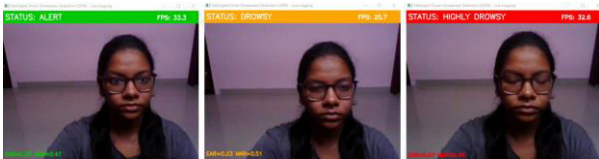
Fig-2: Live Detection Output - Alert (EAR≈0.37), Drowsy (EAR≈0.23), Highly Drowsy (EAR≈0.07)
