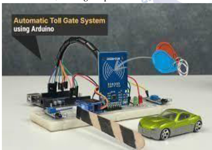
Fig 2.1 RFID Based Access Control System
