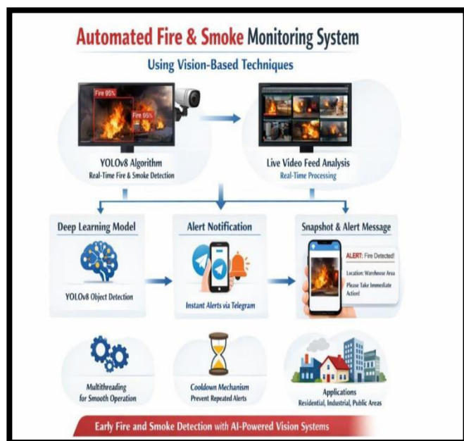
Fig 1: Automated Fire and Smoke Monitoring System
