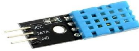
Fig 1.5 DHT11 TEMPERATURE & HUMIDITY SENSOR
