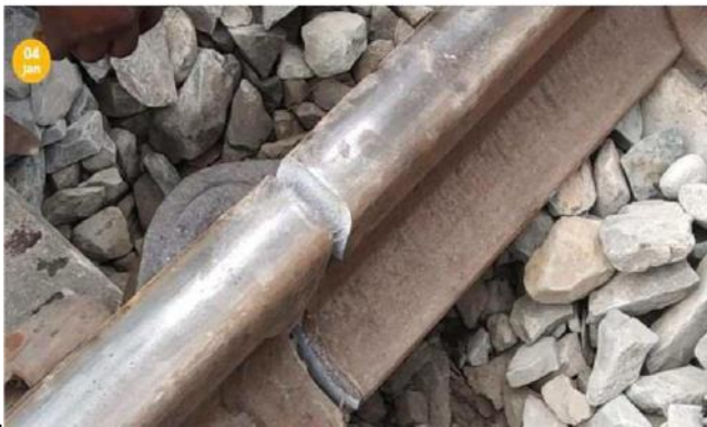
Fig. 2 Part of the track which has a Crack
