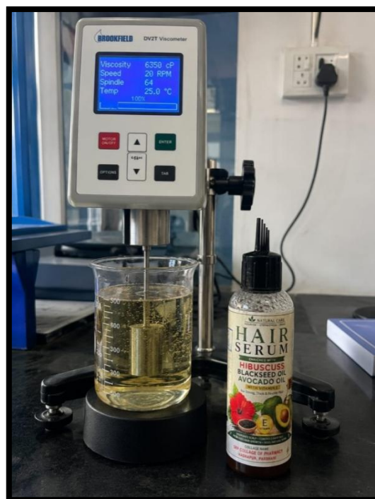
Fig 4. Viscosity Test (Viscometer).
