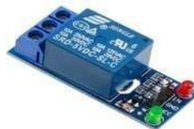
Fig - 5: Relay Module
