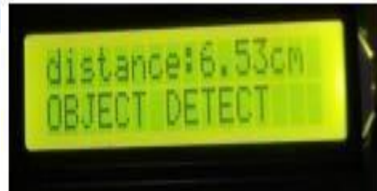
Fig 4.3: Object detected by Ultra Sonic Sensor
