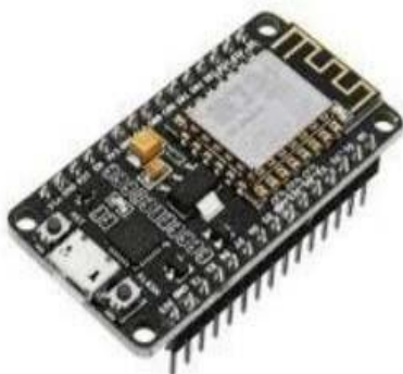
Fig. 4.4: NodeMCU with integrated ESP8266
