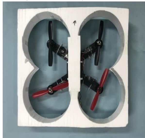
Fig. 1. Top view of the developed drone system installed with guard plate for adhering function
