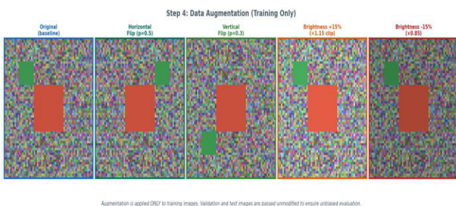
Augmentation is applied ONLY to training images. Validation and test images are passed unmodified to ensure unbiased evaluation.
