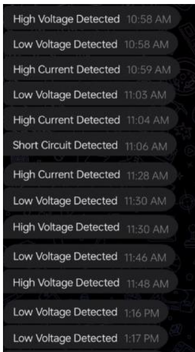
Fig. 13 Telegram notification of fault detection
