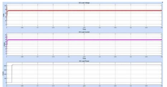
Fig. 9: Output wave forms of online MPPT technique (Incremental Conductance)
