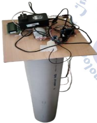
Figure 4. Prototype implementation of the IoT-based borewell child rescue system showing the ESP32 controller, sensor modules, robotic gripper, and oxygen supply unit.
