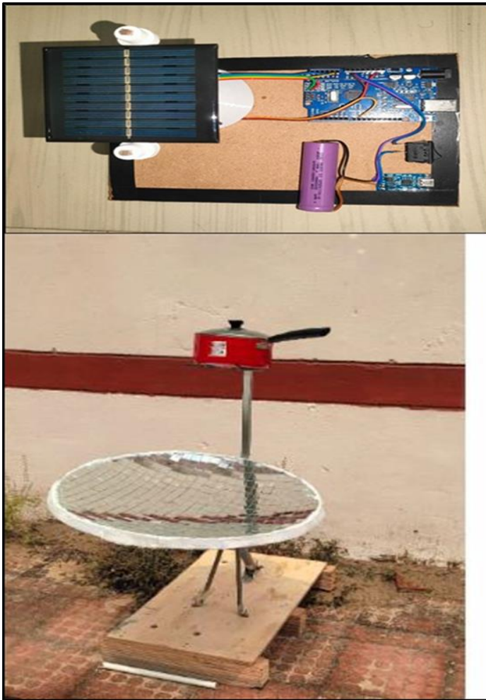
Fig. 5. Integrated experimental setup showing Arduino-based tracking subsystem and parabolic solar cooker with mounted cooking vessel System performance was assessed in both manual alignment (where the dish was set at the start of the test) and automatic tracking modes. This was done by boiling 1.0 kg of water and recording the cooking time, maximum vessel temperature, average thermal power, solar-to-thermal efficiency, tracking accuracy, shadow losses, and heat retention after cooking. Measurements were taken using calibrated pyrometers, thermocouples, and balances. We repeated the tests over three clear days ( n \geq 3 for each mode) to ensure statistical reliability. What makes this setup different from traditional methods is its tracking logic, lower energy use, reusable package (which includes open-source Arduino code, CAD files, and datasets), and strong experimental protocol that includes
