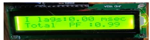
Fig 10: improved power factor after switching to 4 capacitor banks.
