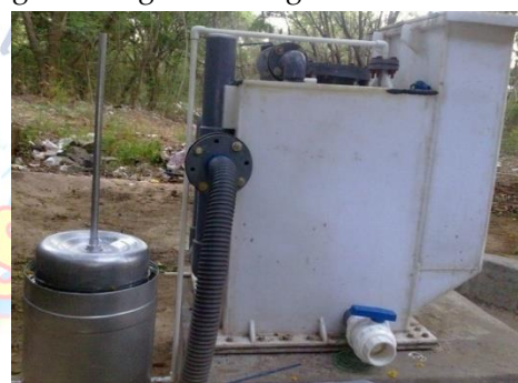
Fig 3 High rate digester using canteen waste
