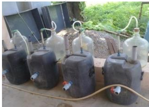
Fig 2 High rate digesters using oilcake
