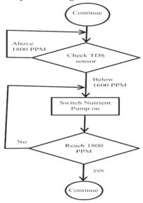
Accurate data helps maintain optimal conditions, preventing crop loss. For instance, if pH exceeds 7.5 or EC surpasses 1800 ppm, nutrient absorption is hindered, potentially harming plant growth.
