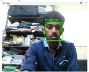
Tests were conducted under various lighting conditions and backgrounds to assess system robustness. The face recognition module demonstrated reliable performance, maintaining accurate identification even with slight changes in facial orientation. Similarly, the sign language recognition module exhibited consistent accuracy across different hand gestures, with real-time speech synthesis providing immediate feedback.
