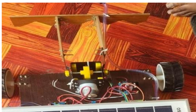
Fig.4:-Dripper setup for Plugging purpose (input-12v, Output-45 rpm)
