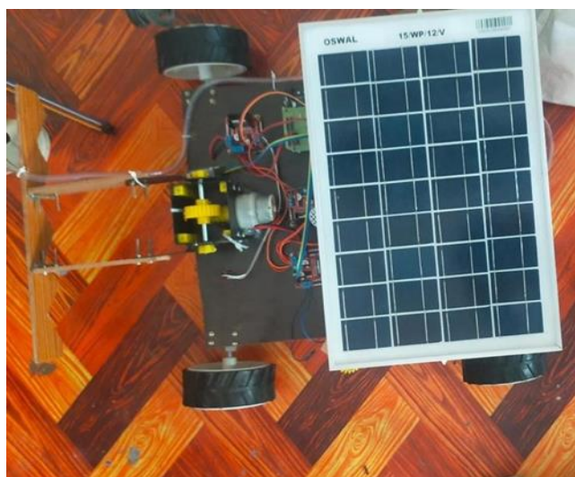
Fig.2:-Final Robot with Plugging, Seeding, Spraying
