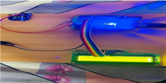
Figure 6: Arduino system in active alert state with LCD and buzzer triggered.
