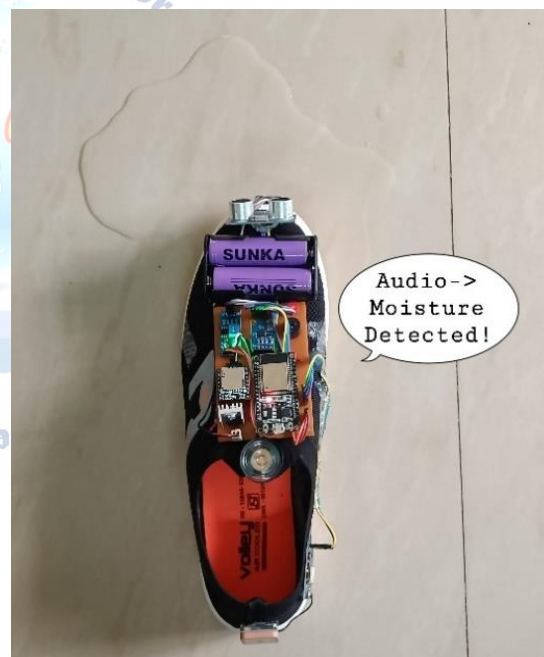
Fig.5: Moisture Detection and Audio Feedback in Smart Shoe
