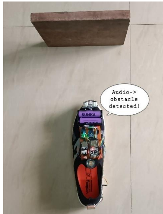
Fig.4: Obstacle Detection and Audio Feedback in Smart Shoe
