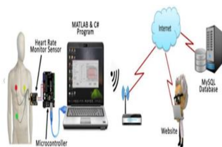
Figure 3. Architecture of the ECG Monitoring System
