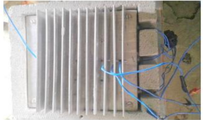
Plate fin array [H=3cm, L=150mm, S=6mm]
