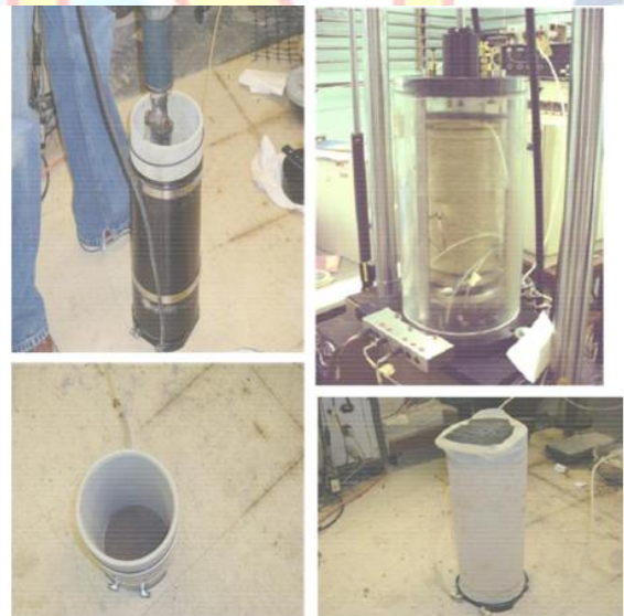
Figure 2.2 Preparation of Testing Limestone Samples.
