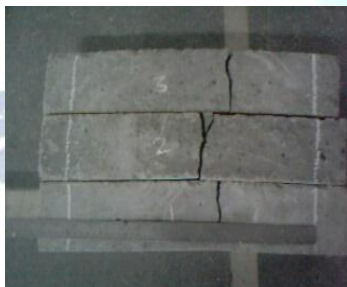
Fig-5 Beams after Flexural strength test
